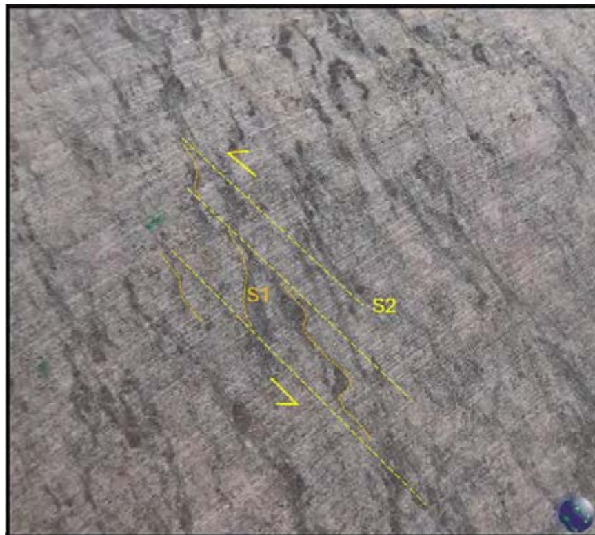
Figure 7.28 S1 and S2 Foliations Developed within Strongly Bleached Magnetite Diorite in the Ghanie Deposit. Photograph from Drill Hole GDD-63 at a Depth of 276.8 m
