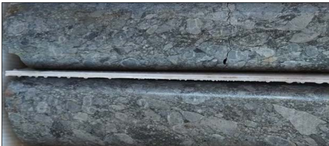
Figure 7.18 An Example of the Conglomerate within the Footwall of the NW Oko Deposit, from 107 m Depth in Drill Hole NWOD-57
