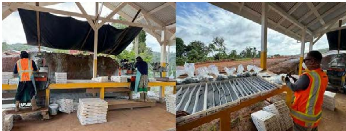
Figure 12.3 Drill Core Cutting and Sampling Process at the Core Logging Facility
