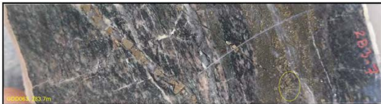
Figure 7.31 Mineralization Associated with Late Pyrite along S3 and S4 Foliations and Veins.
