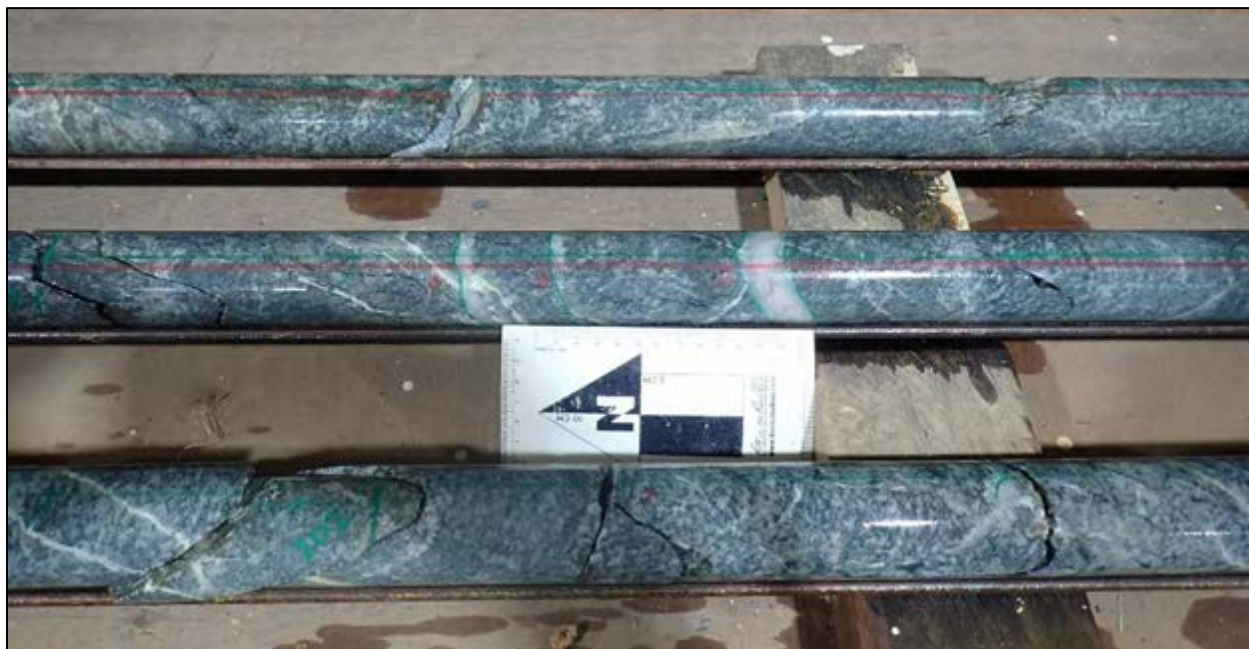
Figure 7.19 An Example of the Ghanie Diorite within the Footwall of the Ghanie Deposit, from 191 m Depth in Drill Hole GDD-190.
