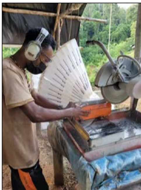
Figure 11.2 Geological Assistant Splitting Drill Core from Hole OKD-97
