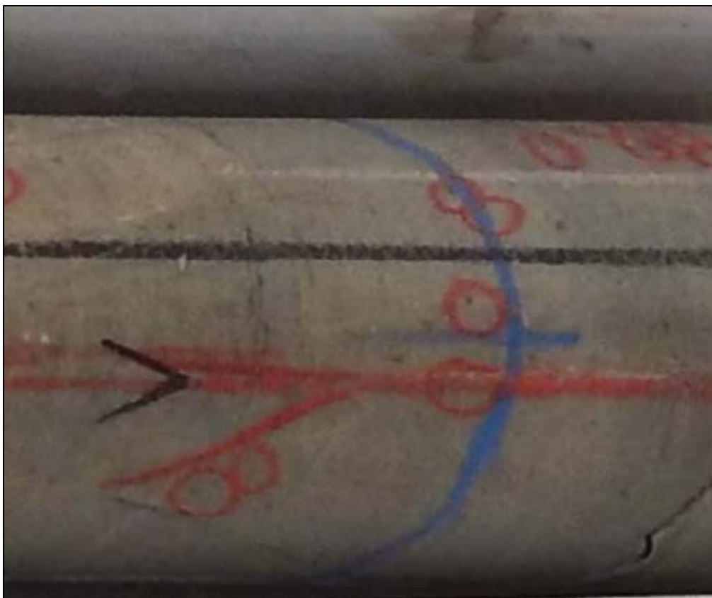
Figure 7.17 Arenaceous Siltstones in the OMZ Deposit, from 81 m Depth in Drill Hole OKD-21
