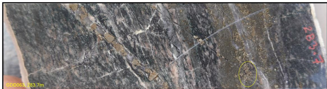
Figure 7.28 Mineralization Associated with Late Pyrite along S3 and S4 Foliations and Veins.
